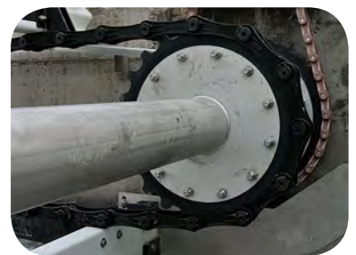
DAF scraper, certified for ex-zone 0
