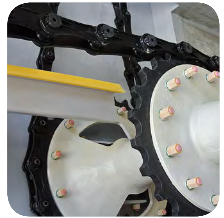
Shaft and flange made from GRP
