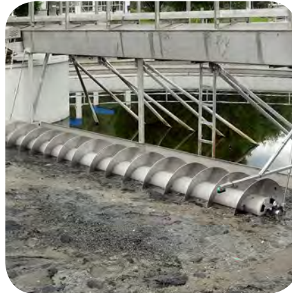
Patented screw conveyor with floating extractor at the side
